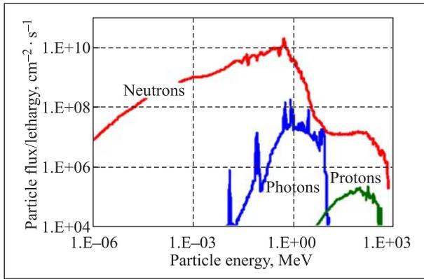
Fig. 5. Neutron, photon and proton fluxes emitted from the assembly under irradiation with 660 MeV protons
