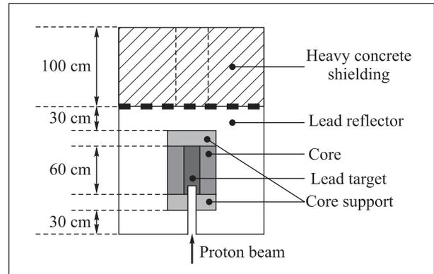
Fig. 6. General scheme of the assembly under investigation
