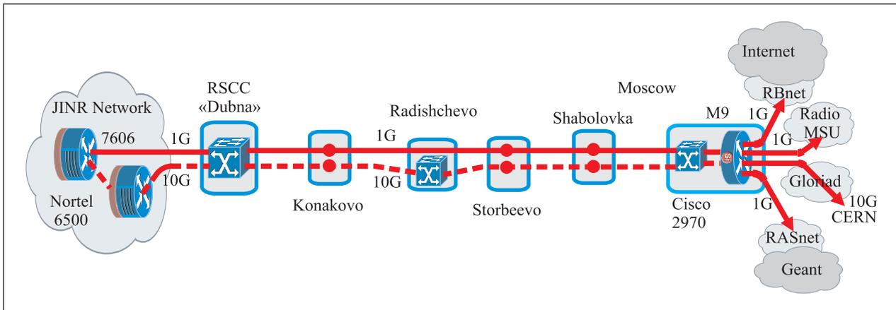
Fig. 1. Scheme of the JINR computer communication links: solid line — operating 1 Gbps channel, dashed line — planned 10 Gbps channel
