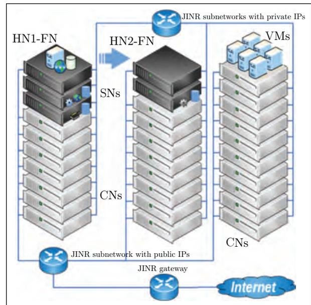
Fig. 6. The scheme of the JINR cloud in configuration of high reliability and availability: HN1-FN, HN2-FN — physical servers with components of the cloud front-end machine (FN), CNs are cloud working nodes on which the virtual machines (VMs) are placed; SNs — data store units
