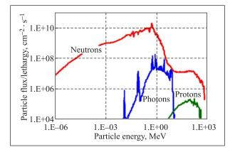
Fig. 5. Neutron, photon and proton fluxes emitted from the assembly under irradiation with 660 MeV protons
