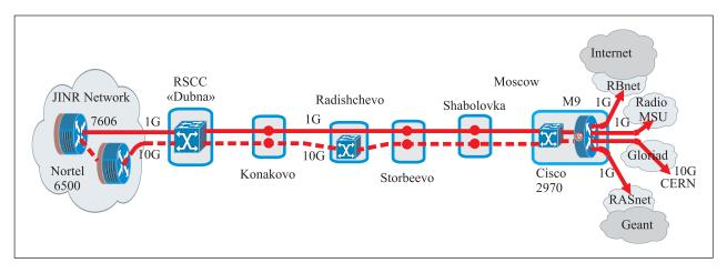
Fig. 1. Scheme of the JINR computer communication links: solid line — operating 1 Gbps channel, dashed line — planned 10 Gbps channel
