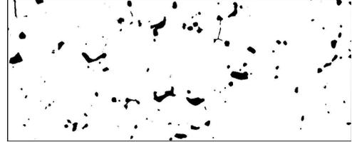
Figure 4: Black-and-white representation of the microphotograph of the surface of an as-polished sample for 16.2 GWd/tM burn-up degree 16.2 GWd/tM
