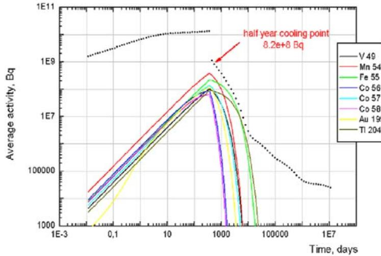
Fig. 3: Activity of the lead blocks surrounding the target as well as isotopes the most active after half a year since the shut down of the SAD
