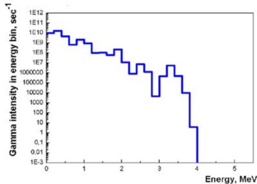
Fig. 4: Gamma intensity in the energy bin (gamma quanta with energy in the limits of one bin of the histogram) in the target ( $\Omega$ )
