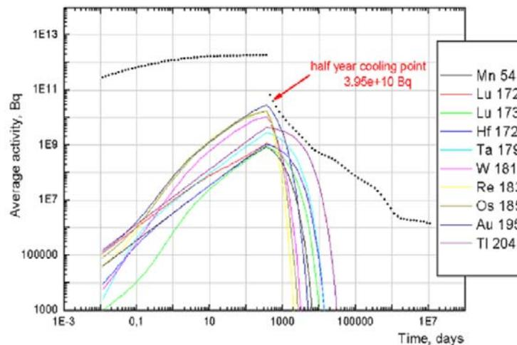
Fig. 2: Total activity of the lead target as well as isotopes the most active after half a year since the shut down of the SAD
