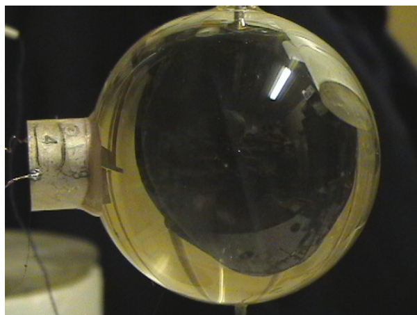
Fig. 2: Sonoluminescent bubble in the center of acoustic resonator, diameter \approx 7.5 cm, filled with degassing water (Institute in Physical-Technical Problems, Dubna)
