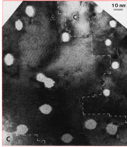
Fig. 1: High-resolution image of Au 24+ -irradiated YBa 2 Cu 3 O 7 thin film [4] (see text)
