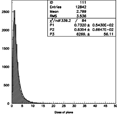
Figure 2: Approximation of the distribution of pion energy losses in the TRD prototype by a log-normal function (2)
