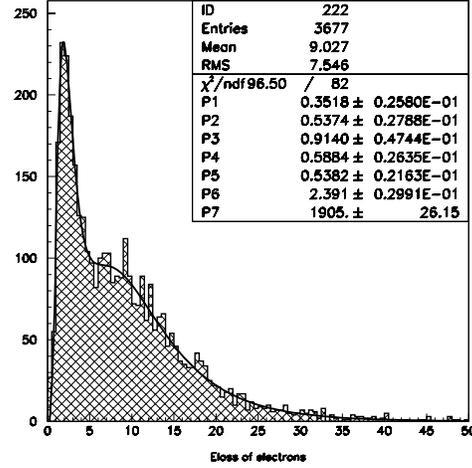
Figure 3: Approximation of the distribution of electron energy losses in the TRD prototype by a weighted sum of two log-normal functions (3)
