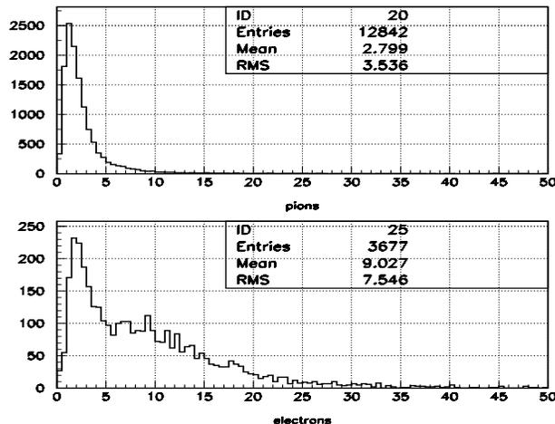
Figure 1: Distributions of energy losses of  $\pi$  (bottom plot) and  $e$  (top plot), including the transition radiation, in the TRD prototype:  $p = 1.5$  GeV/ $c$
