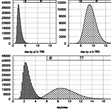
Figure 5: Distributions of variable  $\overline{\Delta E}$  for  $e$  (left top plot),  $\pi$  (right top plot); summary distribution (bottom plot)
