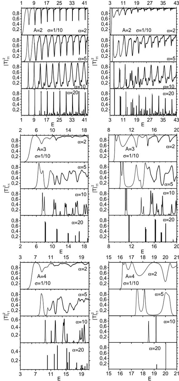
Fig. 6. The total probabilities of transmission through the repulsive Gaussian barriers for the system of  $A = 2, 3, 4$  particles, coupled by the oscillator potential and being initially in the ground symmetric (left) or antisymmetric (right) state, vs the energy  $E$  (in osc.u.).
