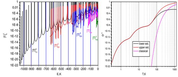
Fig. 9. The total probability of penetration from all 5 channel with energies (in K) to all five open channels, and the diffusion coefficient or thermal rate constant vs. temperature. Comparison with the classical diffusion coefficient.
