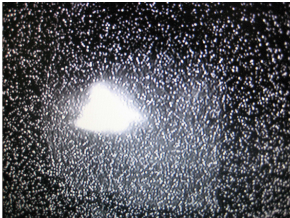
Fig. 2: The photo of the extracted proton beam profile at the exit from the AIC-144 cyclotron in the experiment of 17 July 2012.
