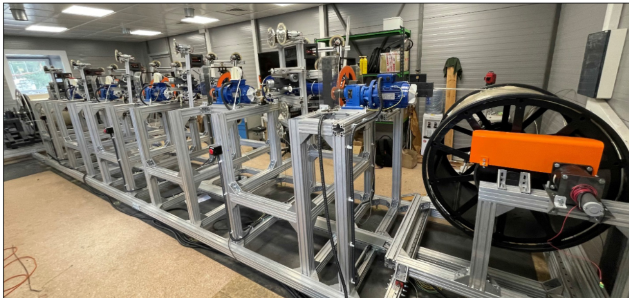
Figure 23. High-current HTS cable winding machine.
