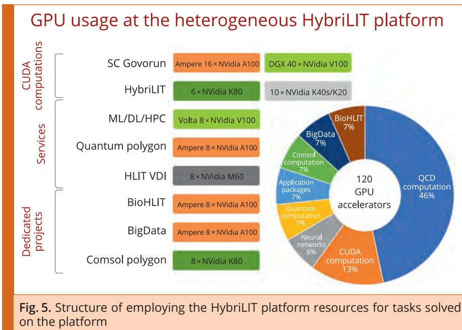
proach [3, 5]. The structure of utilizing the graphics accelerators of the HybriLIT platform is displayed in Fig. 5.
