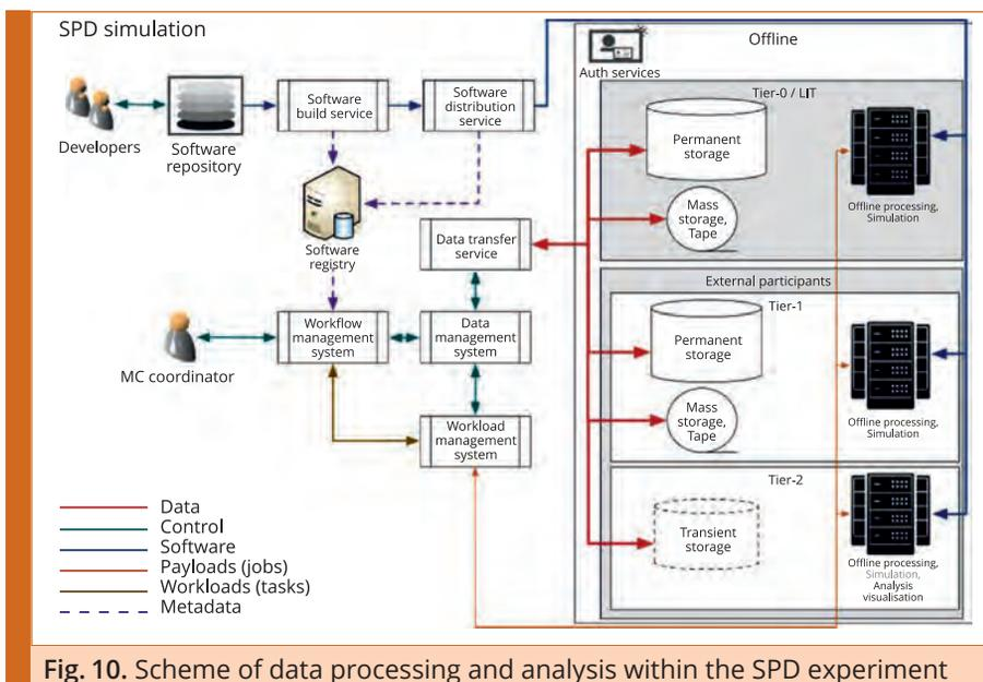
Fig. 10. Scheme of data processing and analysis within the SPD experiment
