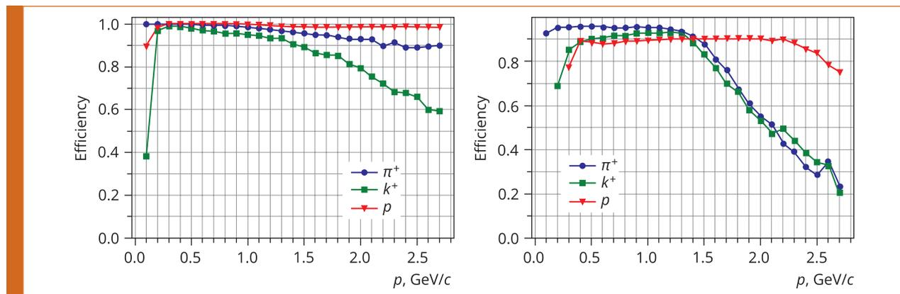
Fig. 9. Effectiveness of charged particle identification in the MPD experiment. Using the gradient boosting method (XGBoost) (left), using the n-sigma method (right)
