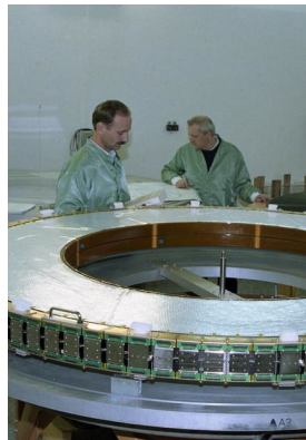
The eight-layer module of the TRT ATLAS transient radiation detector is being tested before being sent to CERN (photo.jinr.ru)
