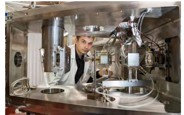
The picture shows the calibration of charged particle telescopes at the ACCULINNA-2 facility. In the photo A.A.Bezbakh (photo.jinr.ru)
