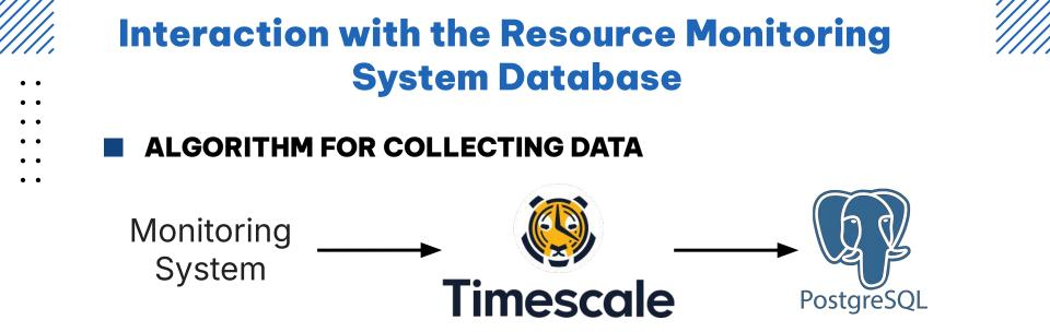
For each node of the computing cluster, data with different periods are regularly taken from the TimescaleDB: for the last week, month and year. This data is then written to PostgreSQL at 5-minute intervals. After that, they are unloaded from PostgreSQL and sent to DataLens for visualization.
