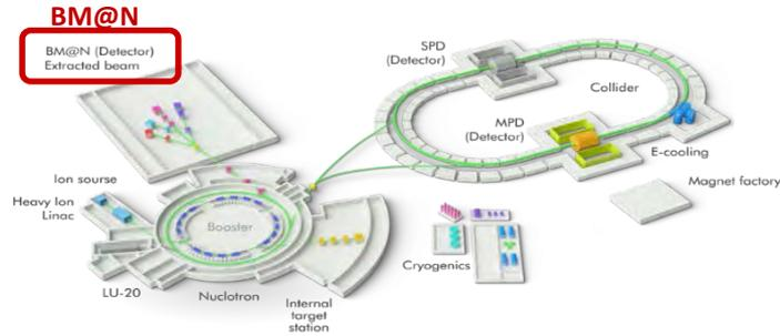
NICA (Nuclotron-based Ion Collider fAcility) accelerator complex located at Joint Institute for Nuclear Research in Dubna
