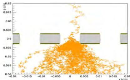
Electron avalanche production from one ionizing electron in a hole (GEM-1 0.6 cm readout)
