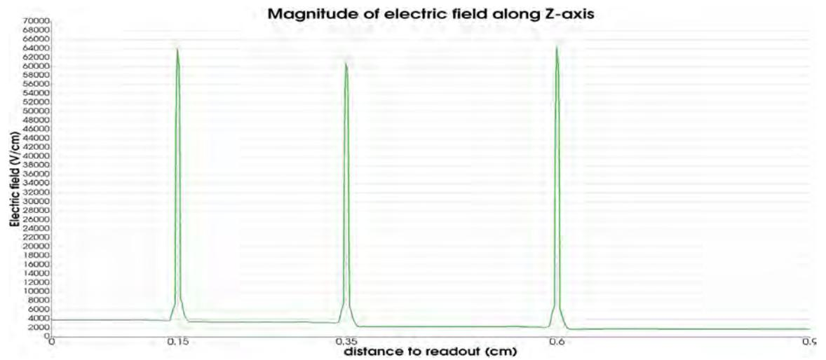
Electric field magnitude *along the line* through the holes with 25 μm shift from the whole thickness of GEM
