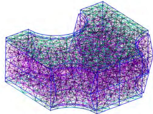
Generated mesh is filled with tetrahedral elements suitable for second-order interpolation that is supported by Garfield++
