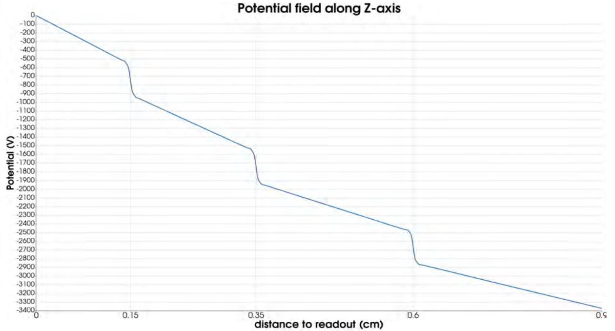
Electric potential magnitude *along the line* through the center of the holes in the whole thickness of GEM
