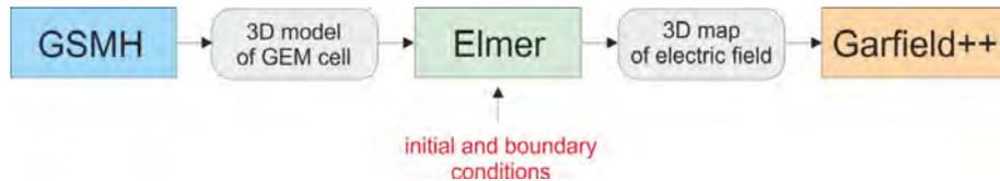
Stages of detailed simulation for the GEM detector
