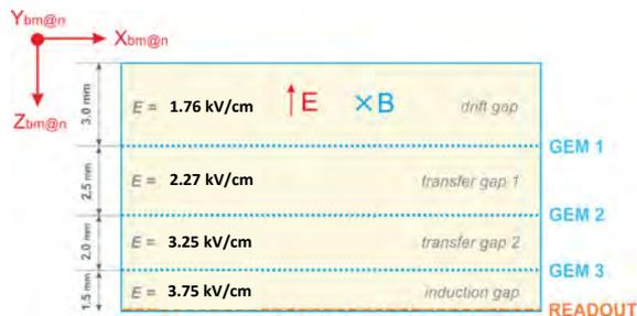
We use Garfield++ for detailed simulation of physics processes in our GEM chamber:
