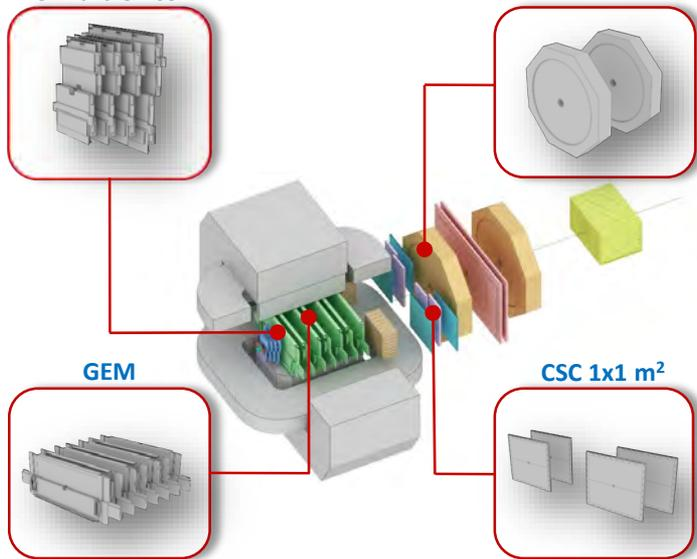
Tracking detectors of the BM@N setup for RUN-8
