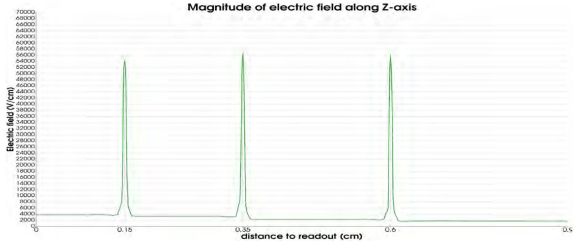
Electric field magnitude *along the line* through the center of the holes in the whole thickness of GEM
